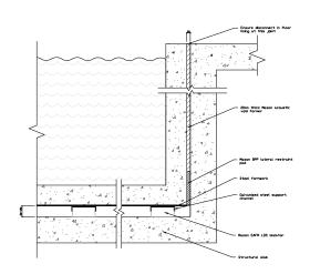
PD TYPICAL DETAIL - EAFM POOL ISOLATION 01 NTS - Steel Formwork
