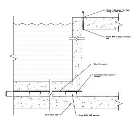
PD TYPICAL DETAIL - EAFM POOL ISOLATION 05 NTS - Steel Formwork With Alternate Lateral Restraint
