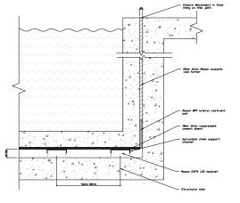
PD TYPICAL DETAIL - EAFM POOL ISOLATION 02 NTS - Compressed Cement Sheet Formwork
