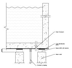
PD TYPICAL DETAIL - EAFM POOL ISOLATION 06 NTS - Steel Formwork on Shear Walls
