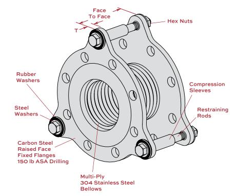
Our steam service ratings are very low in the interest of safety although our 70°F (21°C) pressure ratings are as high or higher then our competitors. All locations where failure could lead to personal injury or suffocation must be avoided. In dangerous locations we suggest housed expansion joints, solid loops, ball joints, packed devices, etc. rather than thin-walled flexible products regardless of manufacturer.
