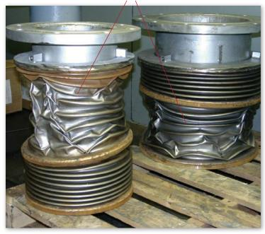
Competitor Pressure Failures.
