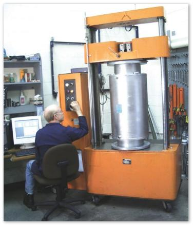
Spring Rate Test in Progress.
