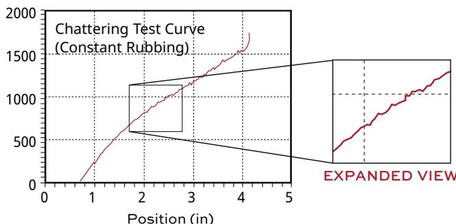
Since there is no need for so small a tolerance, our clearances are roomier for smoother travel, as shown by the Mason test curve below. When expansion joints bind, it increases the anchorage loads. Binding intermediate rings stretch bellows unevenly and can cause failure.
