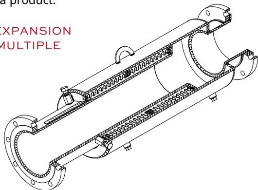
Oddly enough, some people still describe the 2" (51mm) movement Expansion Compensators as internally pressurized. They are not. Only the old design on the previous page is internally pressurized.
