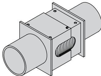
Some years later, there was a major change in concept. The industry turned to a completely housed construction. In this design, the bellows is welded to a sliding flange on the end of
