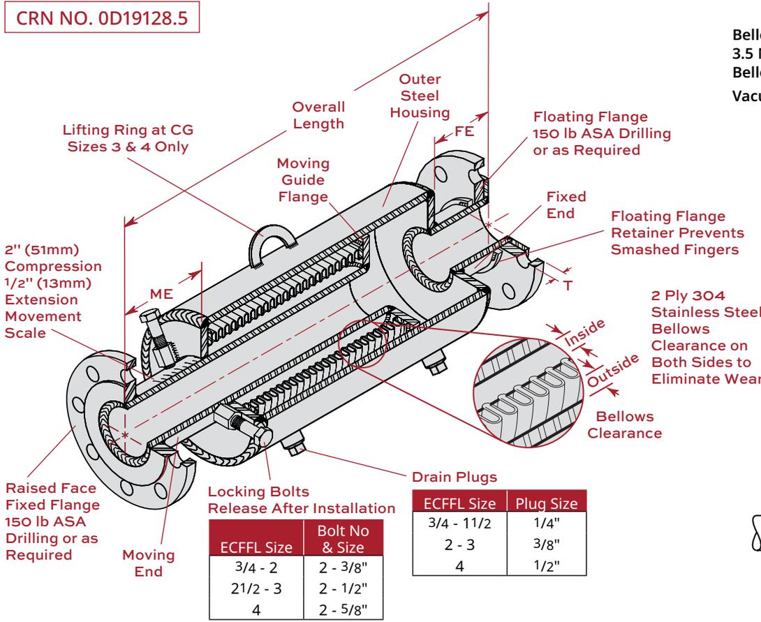
Bellows are externally pressurized.
