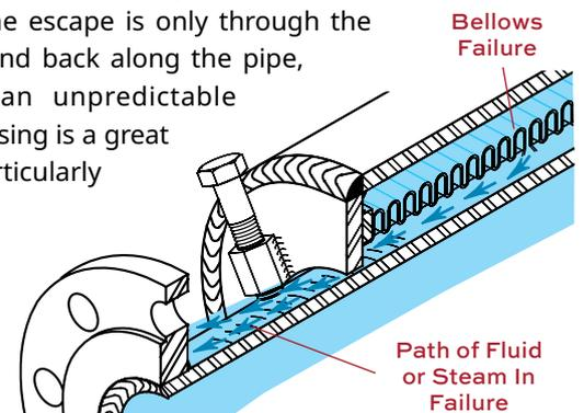
For whatever reason, the entire industry refers to 2" (51mm) movement designs as Expansion Compensators. They are shipped preset to allow for inward travel only in hot lines. Should there be a dual temperature situation, there is no engineering reason the compensator cannot be moved in 3/4" (19mm) before installation, so it would accommodate 1 1/4" (32mm) pipe expansion and 3/4" (19mm) contraction or some other setting.
