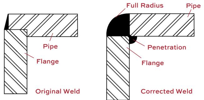
Here again, we checked competitor's products, and found our original technique was typical. We re-examined all of our welds and changed every one to good piping practice with welds as sketched. Maybe this is overkill, but neither you nor we will ever suffer a weld failure again and that's good to know.
