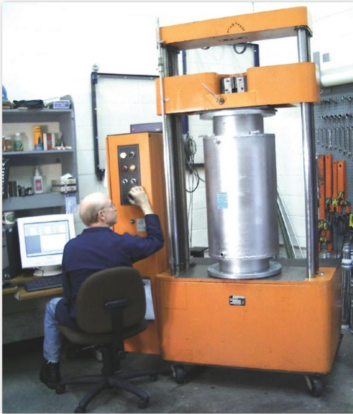
Spring Rate Test in Progress.
