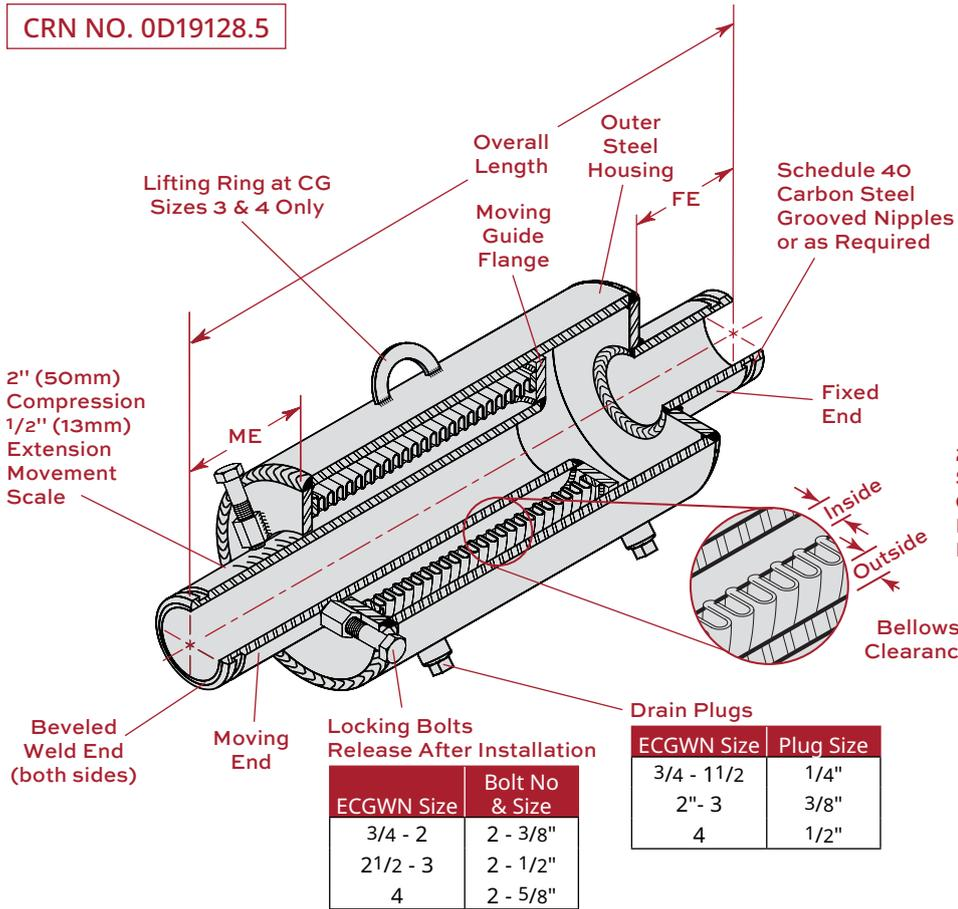
Bellows are externally pressurized.
