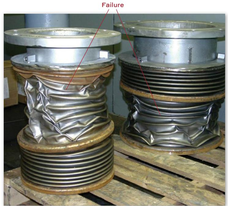
Competitor Pressure Failures.
