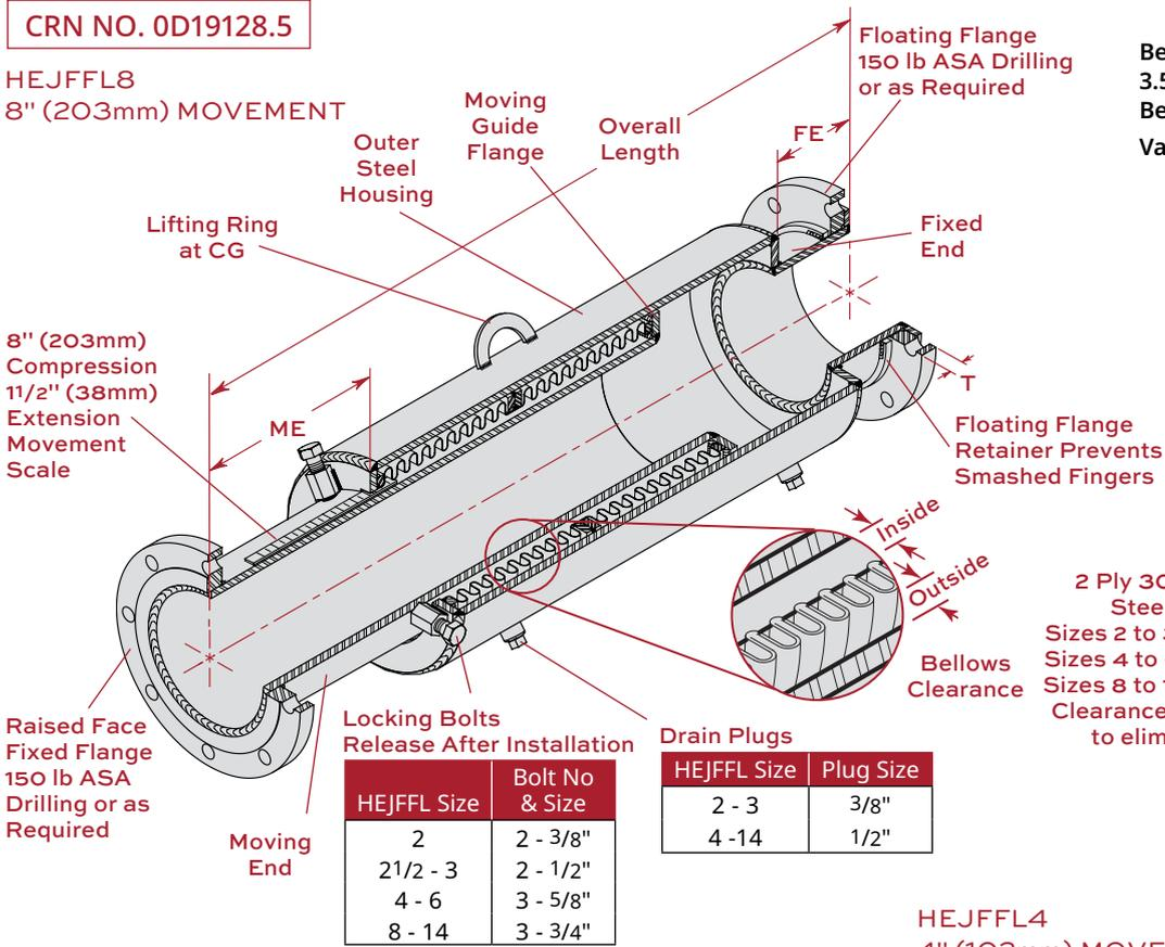
Bellows are externally pressurized.
