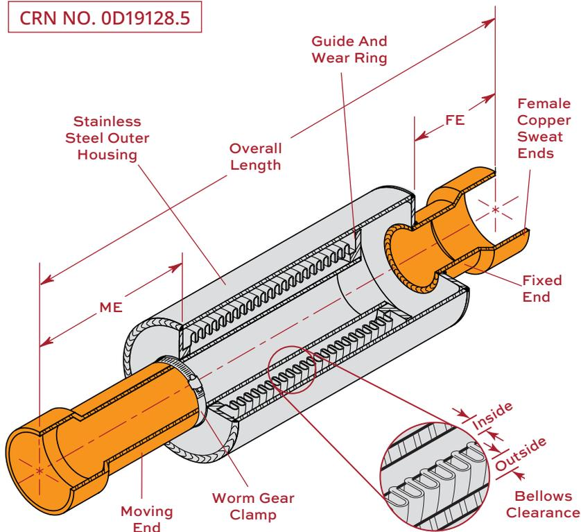
Bellows are externally pressurized. 3.5 Minimum Safety Factor for Both Bellows and Housing.
