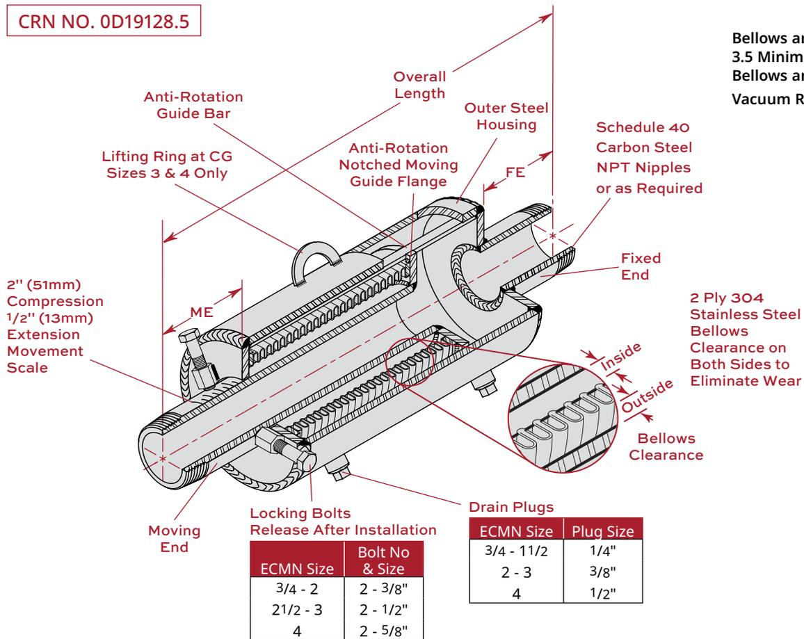
Bellows are externally pressurized.
