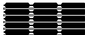
Pads may be stacked with 16 gauge (1.6mm) shims between layers for increased deflection.
