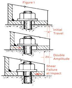
Type HCF Hole Clearance Filler provides a quick solution as it fills this clearance created by practical tolerances, off center bolts or the extreme situation where holes are enlarged on the jobsite by drilling or burning.
