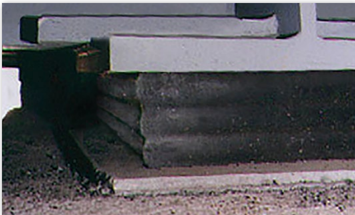
Loaded Bearing Showing Bulges Between Plates
